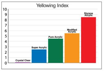
Tests have demonstrated that even acrylic sealers marketed as "nonyellowing" will discolor if subjected to 1,000 hours of QUV testing. This level of testing for yellowing is the equivalent to exposure to Florida sun for over 5 years. CRYSTAL CLEAR continues to be perfectly clear after this test.
